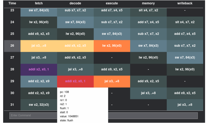
Figure 2: Pipeline rendered as a website
