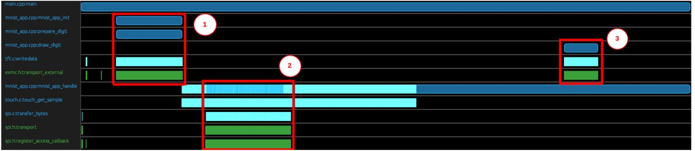
Fig. 6: Annotated FLD of single handwritten digit detection using NN pretrained with MNIST database; blue is SW, green is HW, boxes with border indicate single execution, boxes without border depict multiple executions, color tone indicates execution frequency (the brighter, the more frequent)
